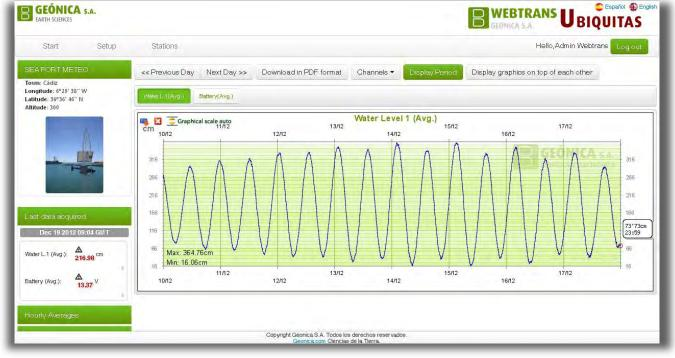
**WEBTRANS** *Ubiquitas* is a WEB application designed by GEO-NICA to manage, query and monitor data collected by the remote automatic stations (Meteodata-2000 and Meteodata-3000).
